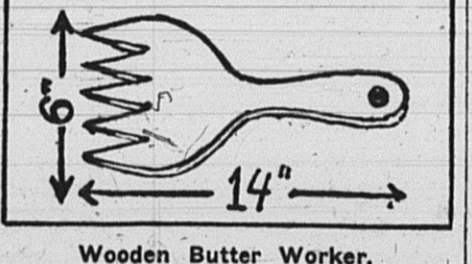
Wooden Butter Worker. help in mixing the salt. It may also be used for taking the butter out of the churn and in working the water out of the butter. Where a big churn is used the fork will be very convenient.
